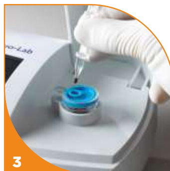
3 Insert Sample tool into cartridge and snap off handle.
