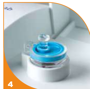
4 Close analyser lid. Result displayed within 4 minutes.
