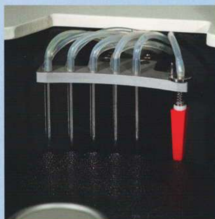
Cuvette-washing units in each reaction tray
